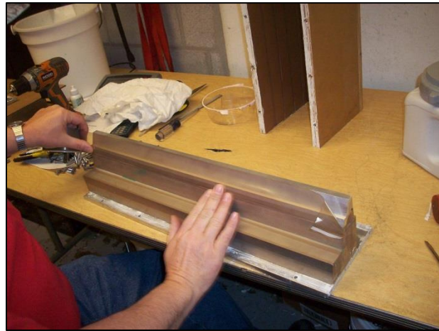
Figure B.2: Application of film tape to leading-edge template.
