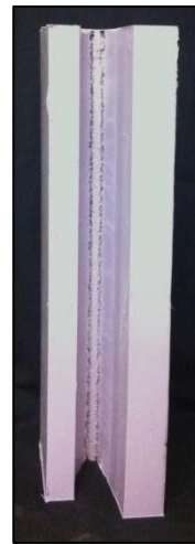
Figure B.24: Completed production mold for horn ice shape.
