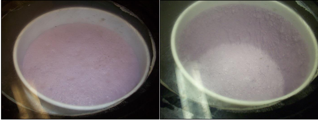
a) b) Figure B.21: Degassing of mold material, a) air is removed from material as it expands and b) most of the air is removed once the material “falls.”
