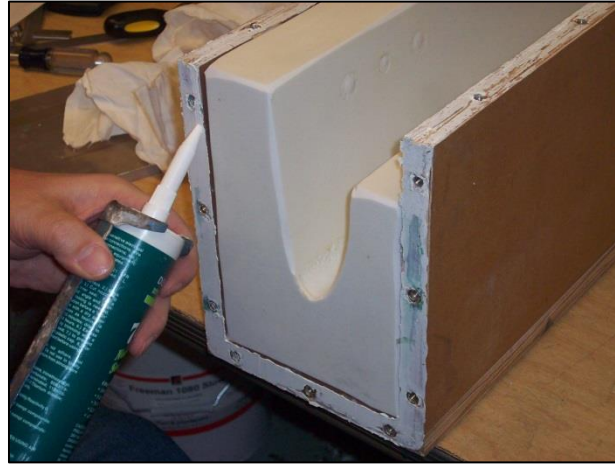
Figure B.4: Application of caulk.
