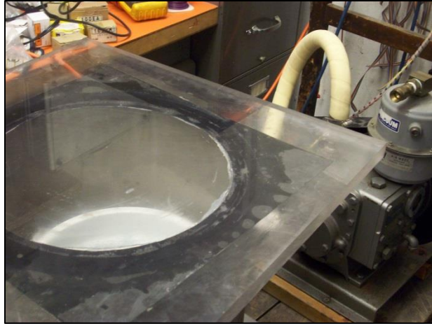
Figure B.10: Casting material inside vacuum pump chamber.
