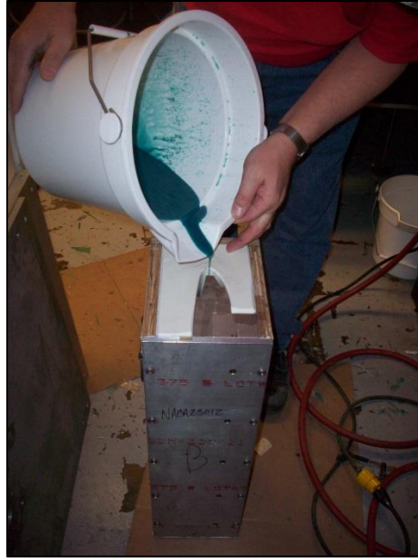
Figure B.12: Pouring of casting material into negative space between mold and leading-edge template to create master casting.
