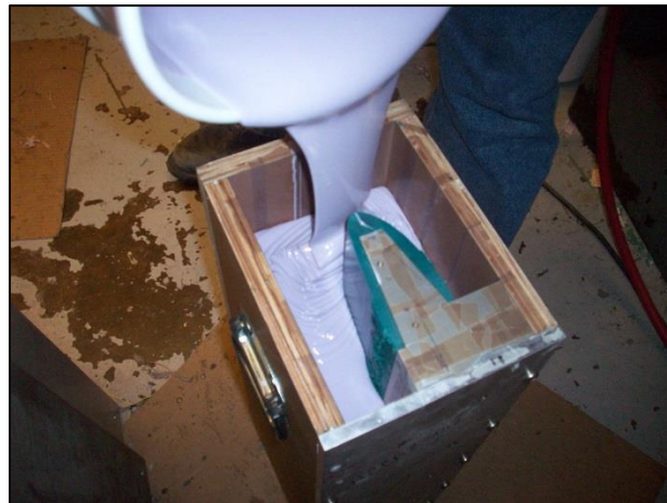
Figure B.22: Pouring of mold material into mold box around master casting.
