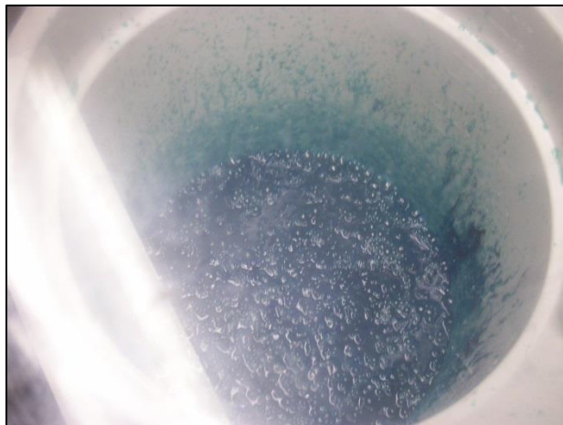
Figure B.11: Removal of air bubbles in casting material in vacuum pump chamber.
