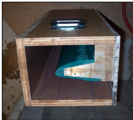
Figure B.18: Master casting in mold box and prepared to make production mold.
