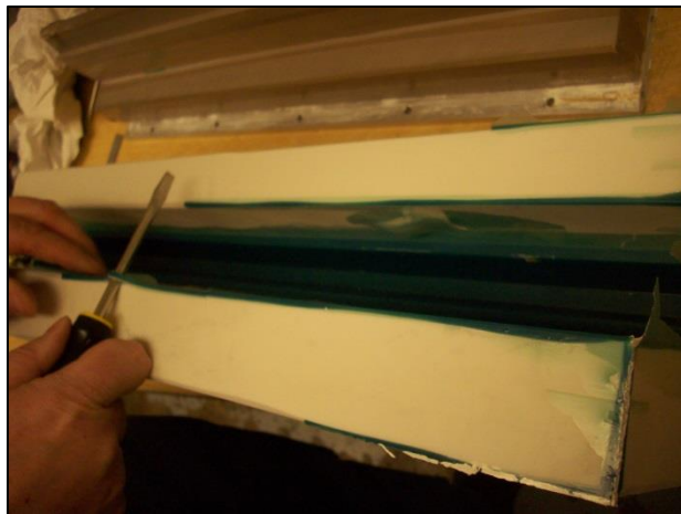
Figure B.15: Removal of master casting from mold.
