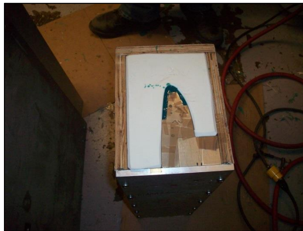
FigureB.13: The casting material left to cure.
