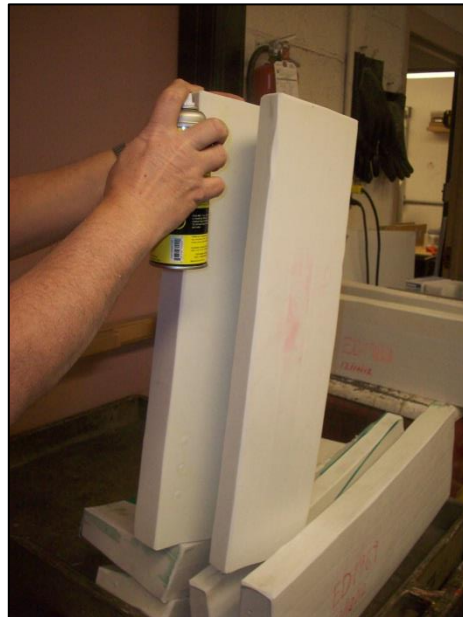
Figure B.3: Preparation of original molds with mold release spray.
