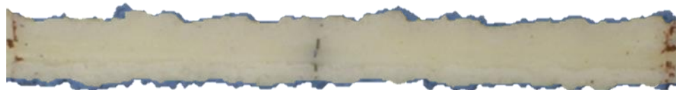
Figure 3.24: Horn ice shapes, casting (top) and RPM shape (bottom) viewed from leading edge with rough location of tips outlined in red.
