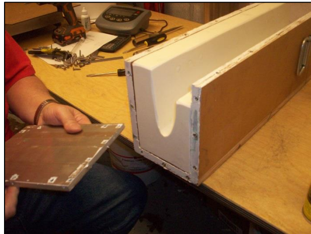
Figure B.5: Placement of mold box bottom.
