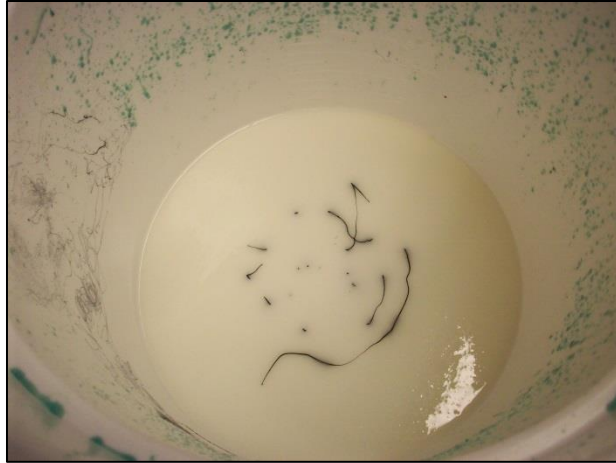
Figure B.8: Typical amount of dye used for each master casting.
